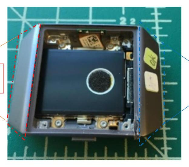
GPS antenna molded to the housing
