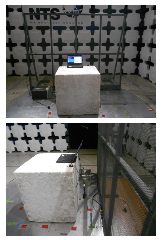
Conducted Emissions Test Configuration Photographs
