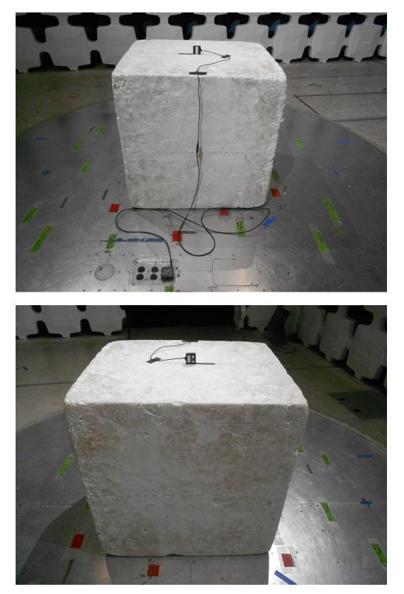
Radiated Emissions Test Configuration Photographs
