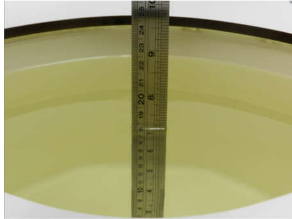
Fig 10.2 Photo of Liquid Height for Body SAR
