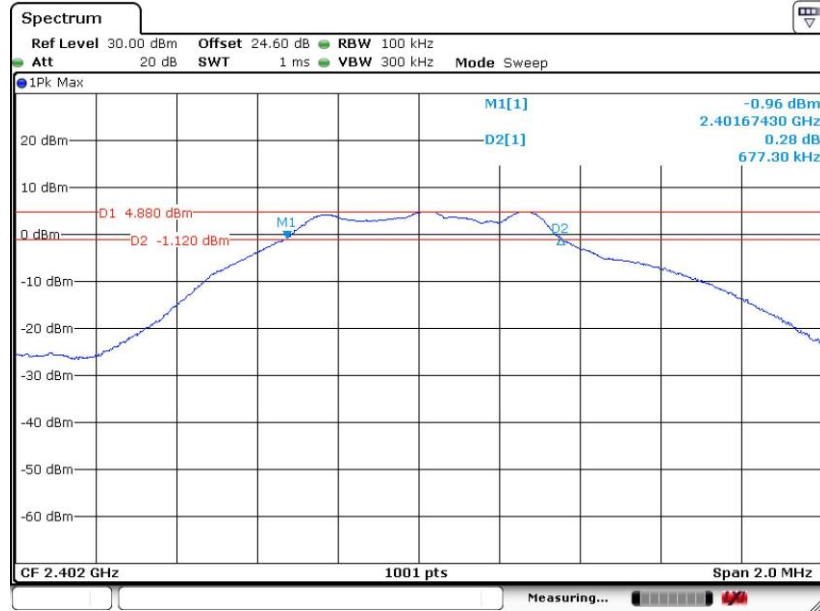
6 dB Bandwidth Plot on Channel 00
