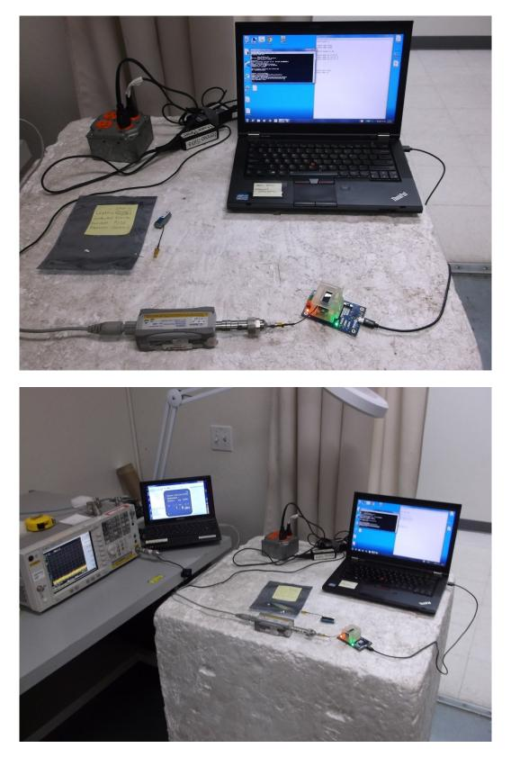
Radiated Emissions Test Configuration Photographs
