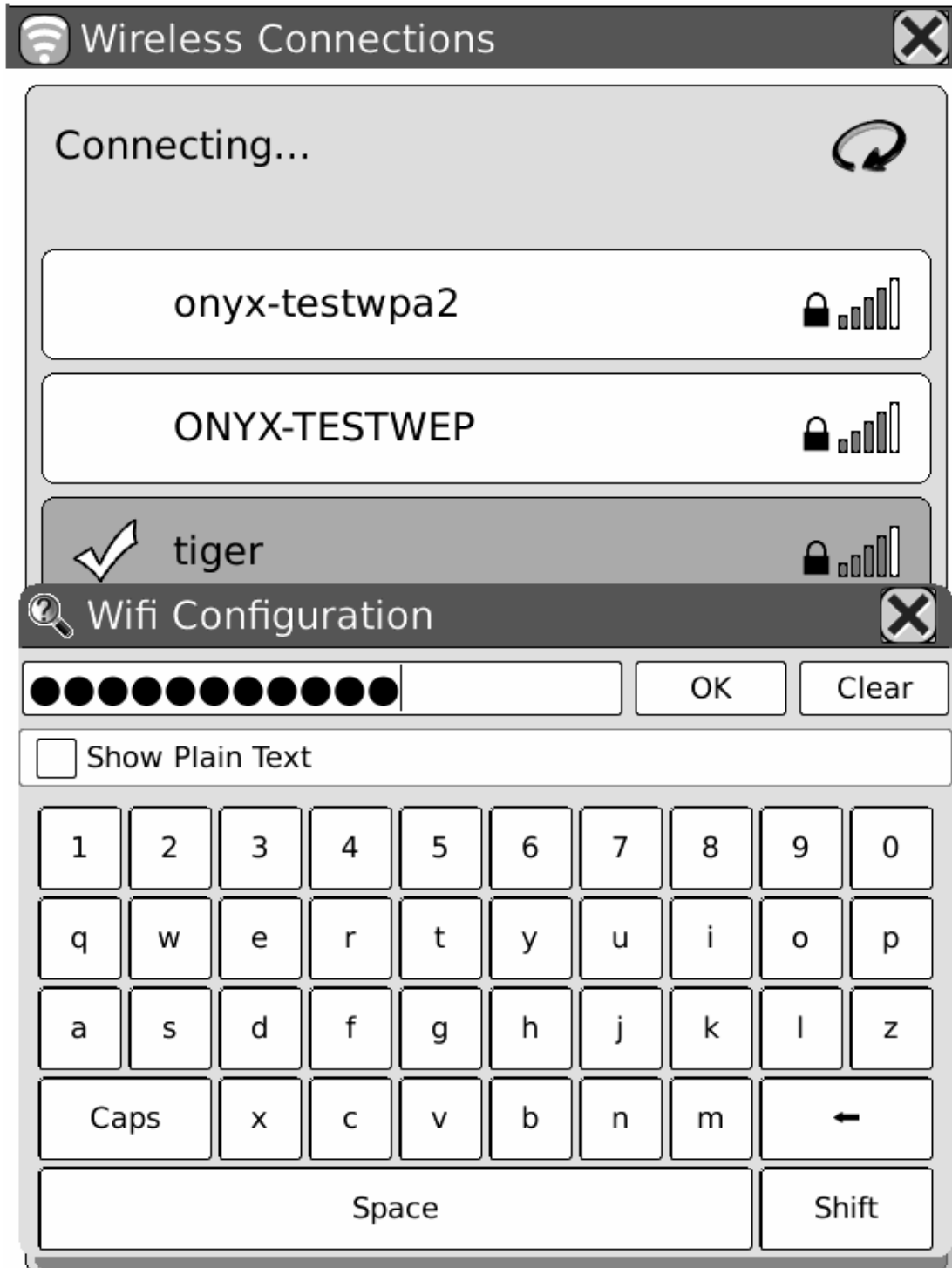
Fig. 6.12.4 Snapshot of Configuring WPA Security Access Point
