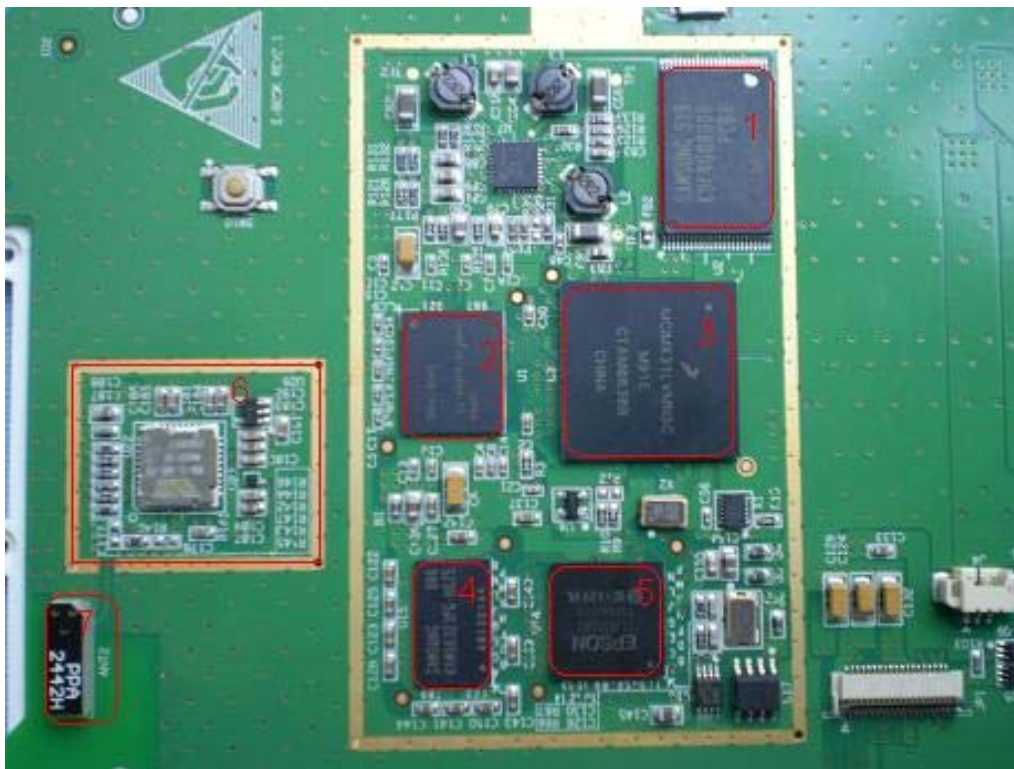
(Note:1. Nand Flash; 2. DDR; 3. CPU; 4.SDRAM; 5. Display Controller; 6.WiFi Module)
