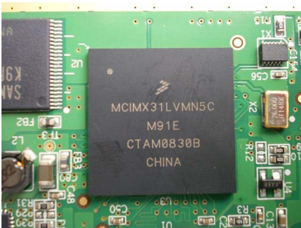
( 3. CPU (Freescale i.MX31L Multimedia Applications Processor) )
