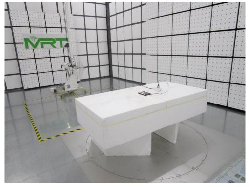
Test Mode: Mode 1/Mode 2 Description: Radiated Emission Test Setup for above 1GHz
