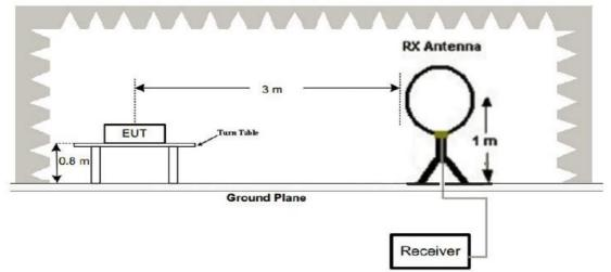
(2) Radiated Emission Test-Up Frequency 30MHz~1GHz
