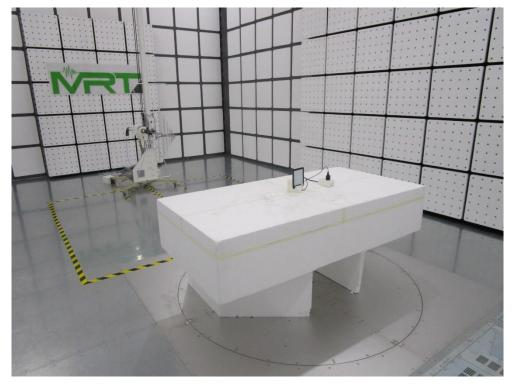
Test Mode: Mode 1/ Mode 2/ Mode 3 Description: Radiated Emission Test Setup for above 1GHz
