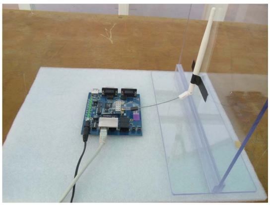
**Radiated Emission Test**
