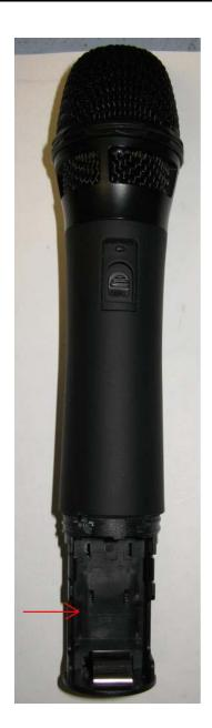
Label will be placed in Battery compartment as shown.
