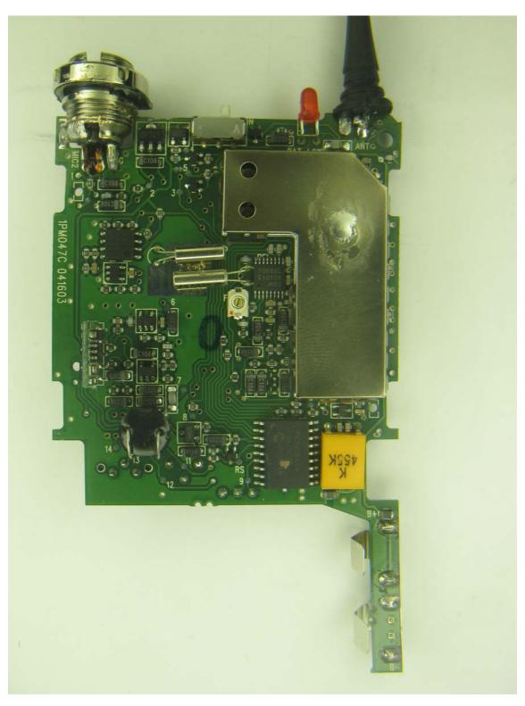
Company: Fender Musical Instruments Corp. Model: UHF WRLS BP Date: January 7, 2010 Photo Description: Component view of PCB
