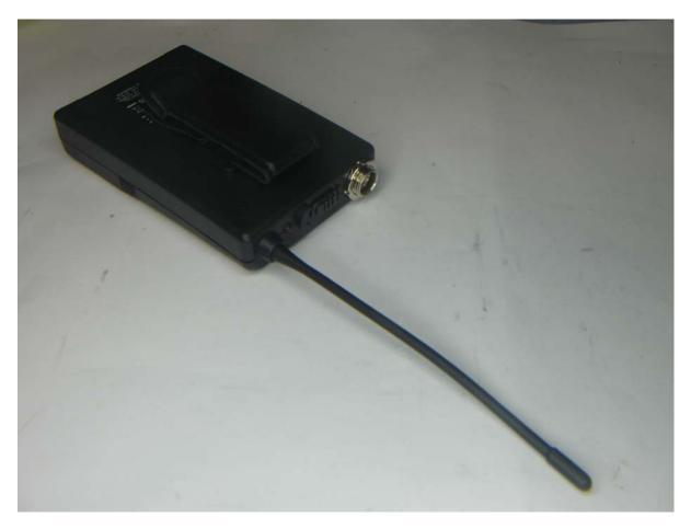
Company: Fender Musical Instruments Corp. Model: UHF WRLS BP Date: January 7, 2010 Photo Description: Transmitter Top View
