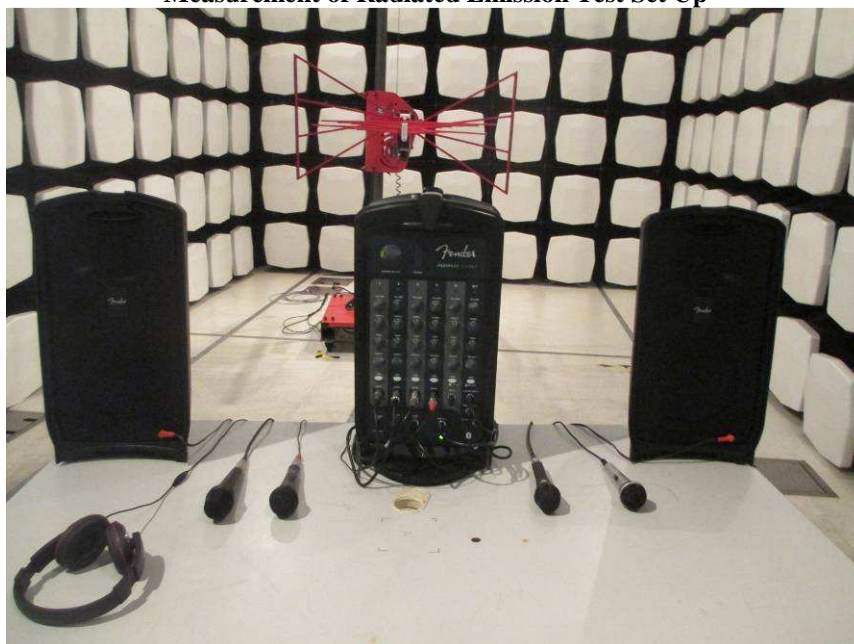
Measurement of Radiated Emission Test Set Up
