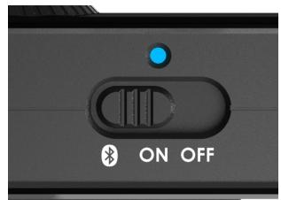
On successful connection, the POWER LED will turn solid blue for 10 seconds and then extinguish.
