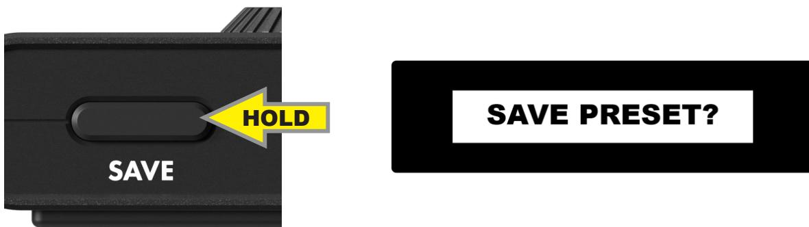
Press the SAVE BUTTON to confirm and save. "PRESET SAVED" will appear in the DISPLAY WINDOW for two seconds; the saved preset name and number will then appear. The display will subsequently time out if no other buttons are pressed:
