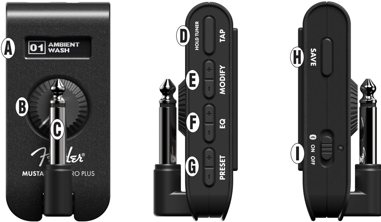
**A. DISPLAY WINDOW:** Black display window with white text shows preset name and number in use. Also displays EQ, MODIFY, SAVE and TUNER functions. To conserve battery life, the display will time out 10 seconds after the last button press; press any button to wake the display.
