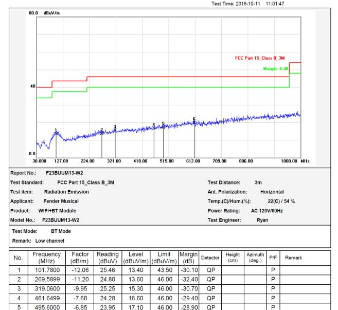
Note: Below 30MHz, the emissions are lower than 20dB below the allowable limit.
