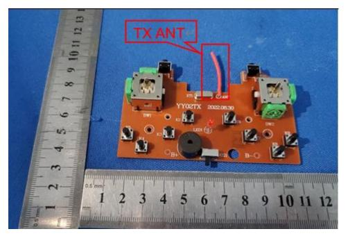
Length: 3cm Antenna Type: Wire Antenna Antenna Gain: 0dBi
