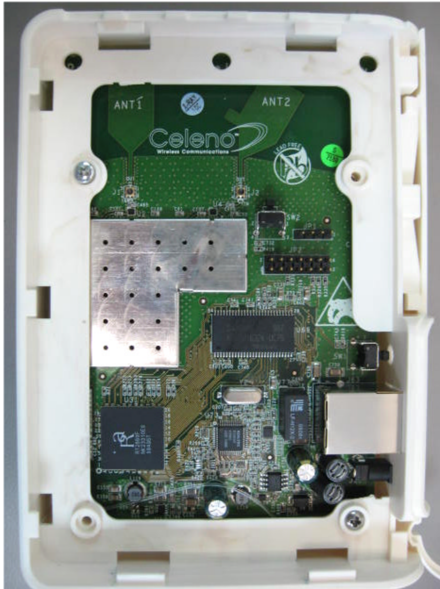
Photograph No.3 Client transceiver internal close view
