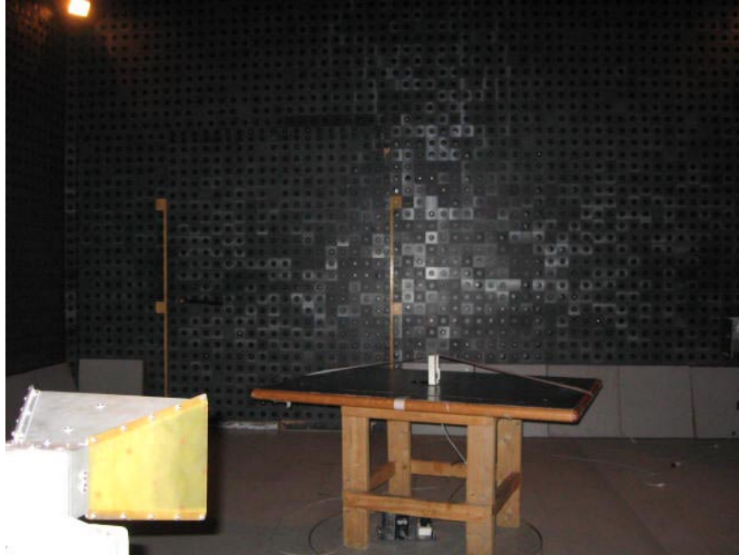
Photograph No.4 Spurious radiated emissions measurement setup in the anechoic chamber above 1000 MHz
