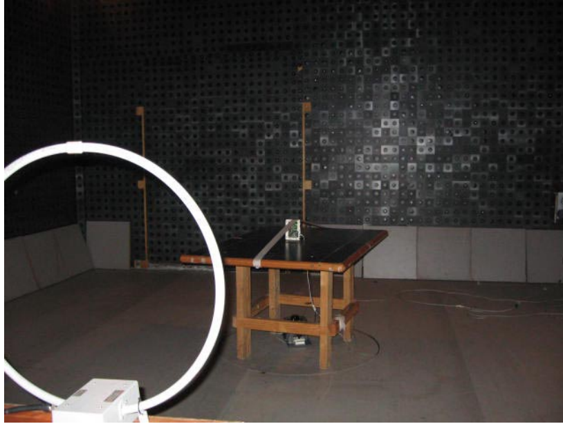
Photograph No.2 Spurious radiated emissions measurement setup in the anechoic chamber below 30 MHz
