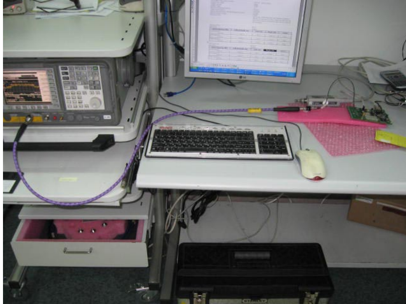
Photograph No.1 Peak output power, peak power spectral density, occupied bandwidth measurement setup
