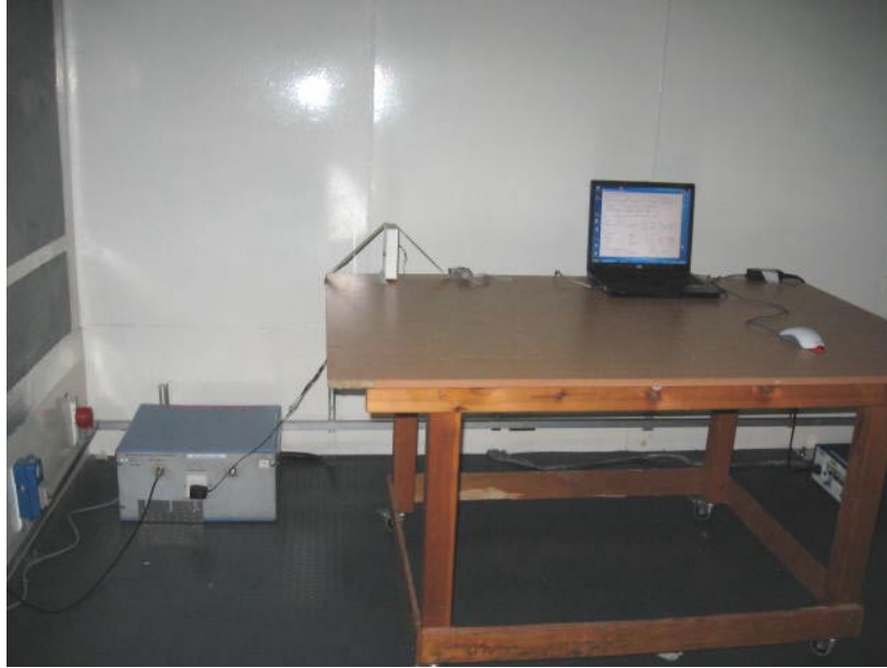
Photograph No.7 Conducted emissions measurement setup
