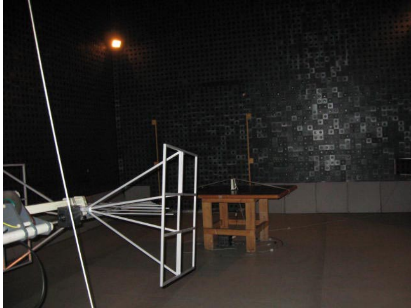
Photograph No.3 Spurious radiated emissions measurement setup in the anechoic chamber in 30 – 1000 MHz
