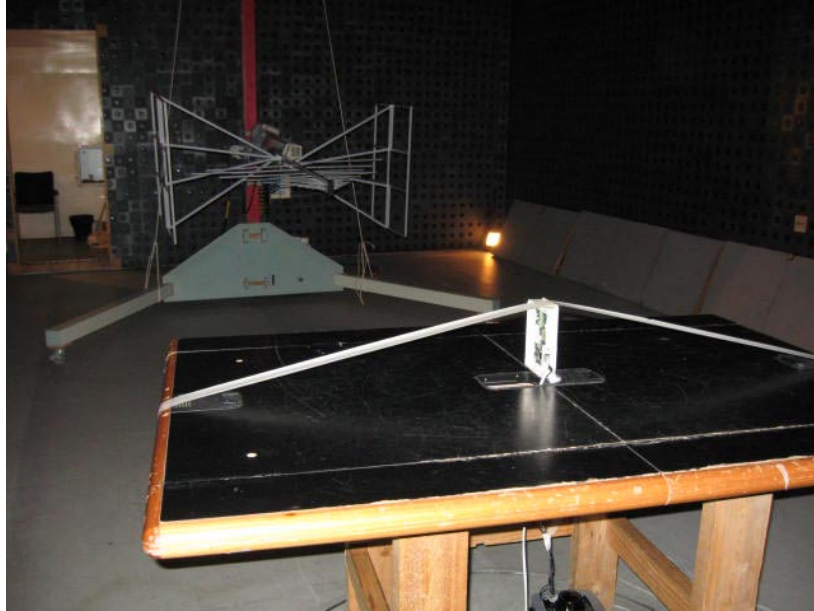
Photograph No.5 Spurious radiated emissions measurement setup in the anechoic chamber, EUT close view
