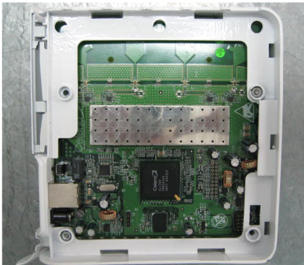
Photograph No.2 Access point transceiver internal view second side
