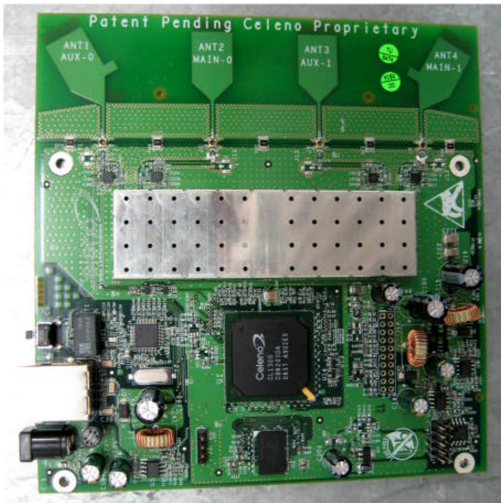
Photograph No.3 Access point printed circuit board front view
