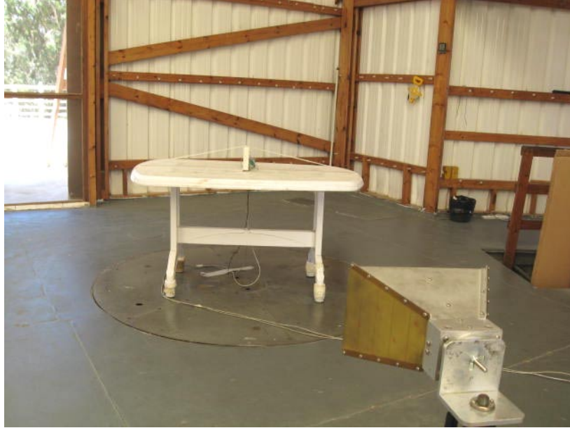
Photograph No.6 Spurious radiated emissions measurement setup at the OATS above 1000 MHz
