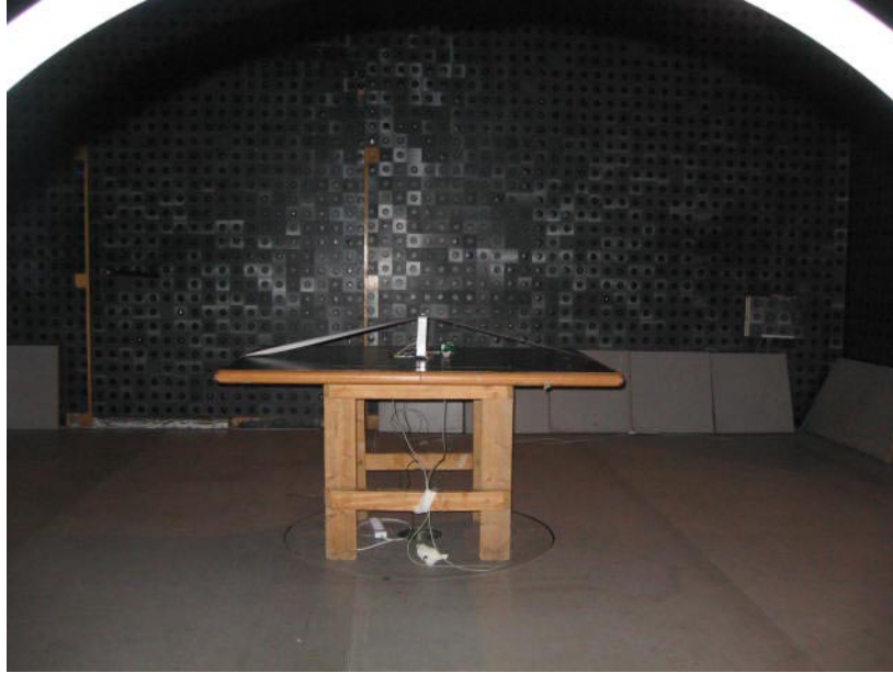
Photograph No.3 Spurious radiated emissions measurement setup in the anechoic chamber below 30 MHz
