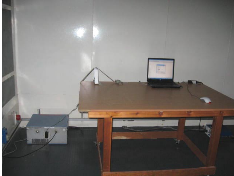
Photograph No.7 Conducted emissions measurement setup
