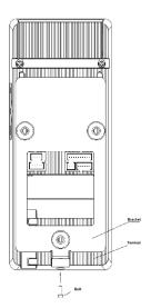
User can drill the holes according to the mounting diagram. Use the 3 wall mount, screws to mount the bracket to the wall.
