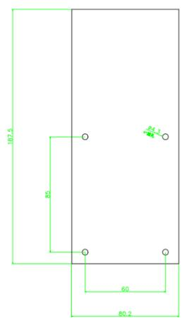
User can drill the holes according to the mounting diagram. Use the 4 wall mount, screws to mount the bracket to the wall.
