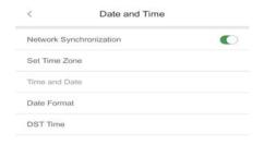
• Date and Time: System date and time can be set with this function. It has the option of syn from the internet or you can turn it off to set the time on device. If you are using the internet time. It is necessary to select the time zone you are in. Otherwise it will have a time difference from the +8 time zone( default time zone is +8)
