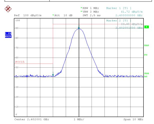
Note:1. Emission level=Read level + Factor. 2. Factor=Antenna factor + Cable loss.
