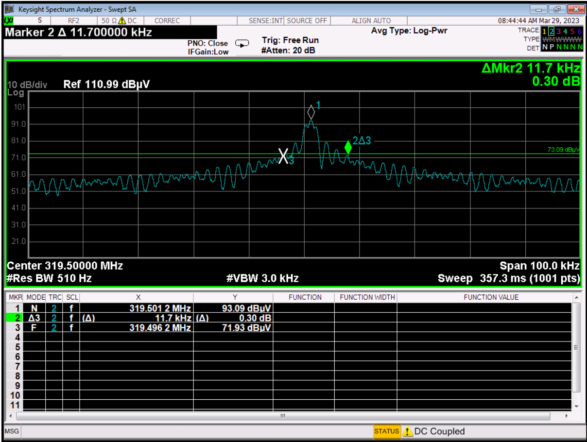
-20 dB Bandwidth Plot – 510 Hz RBW – No External Sensor Adapter
