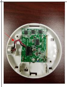
Microphone extended with wires and rubber spacer wrapped around mic.
