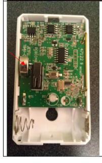
Microphone soldered directly on
