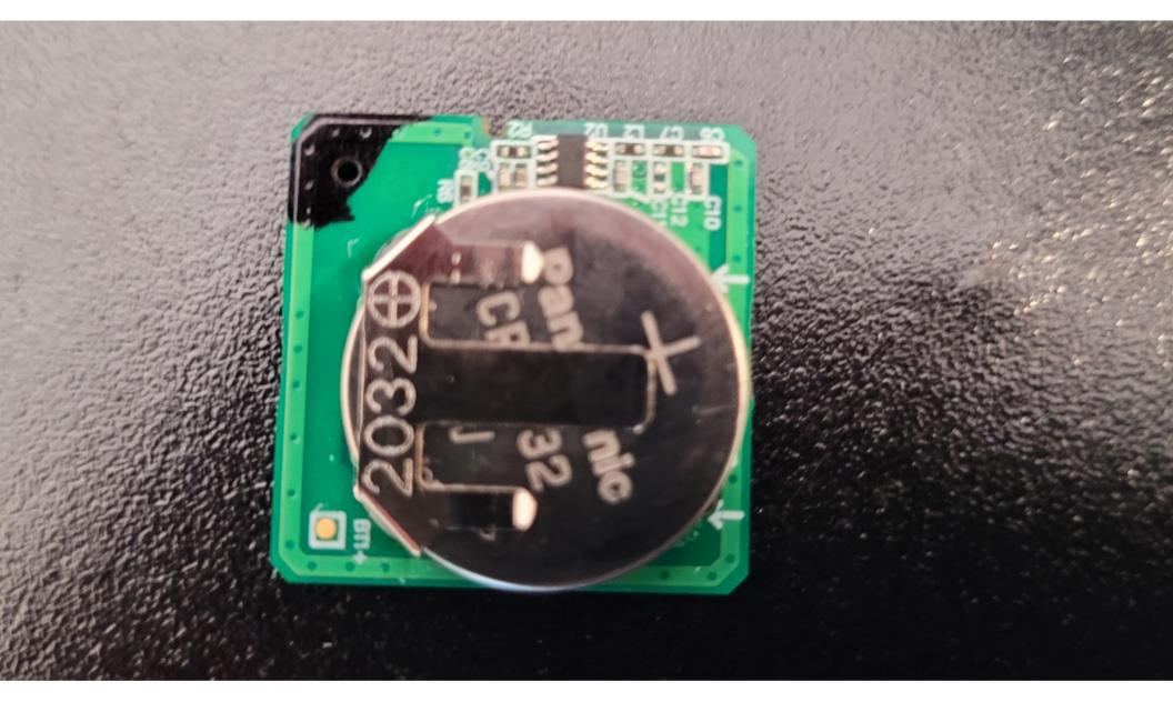
Top View of the PCB with Battery
