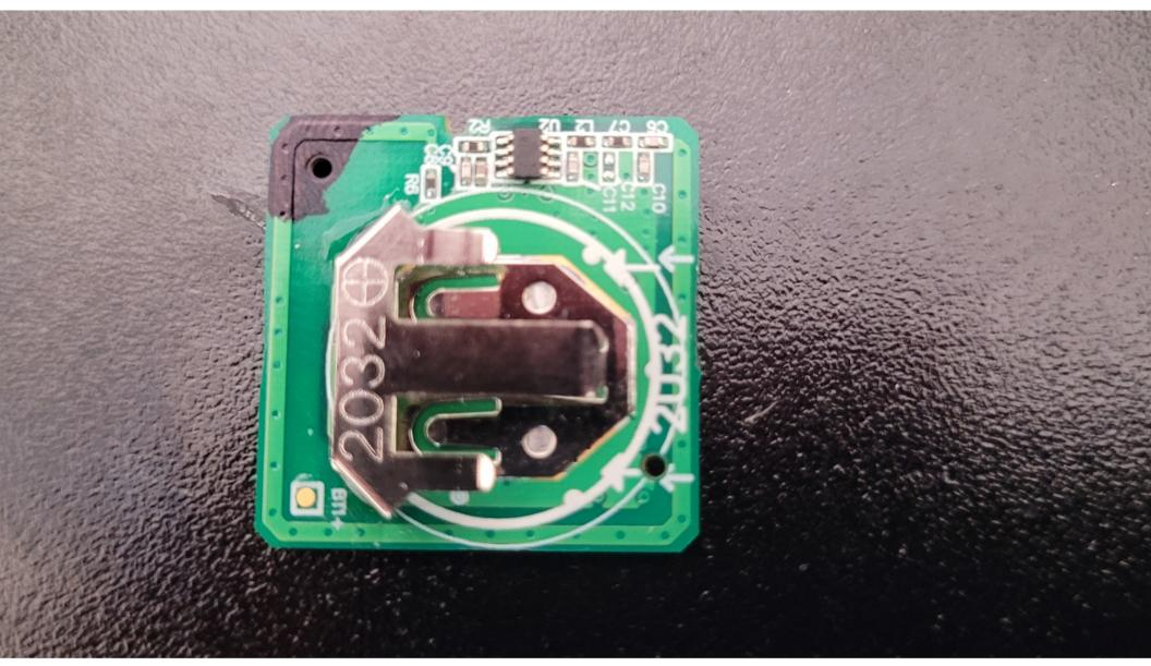
Top View of the PCB with Battery Removed
