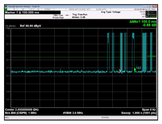
Number of Pulses in worst case 100 ms Each set of pulses has 4 smaller pulses.
