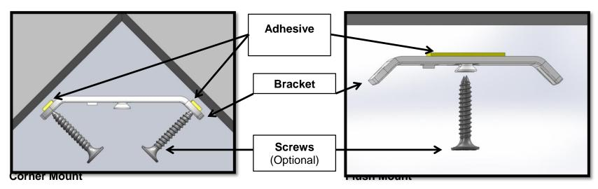
Note: For best results, attach adhesive tape to bracket FIRST, then position on wall. Adhesive tape is VERY STRONG so moving the bracket after attaching will be difficult.
