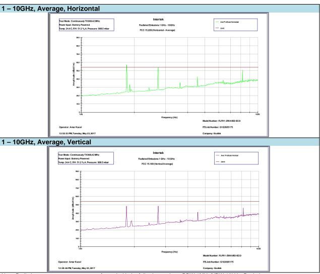
Note: Preliminary average scans were performed with the following settings: RBW 1MHz/VBW 10kHz, Peak detector.
