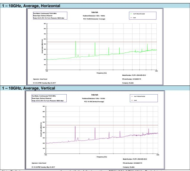
Note: Preliminary average scans were performed with the following settings: RBW 1MHz/VBW 10kHz, Peak detector.
