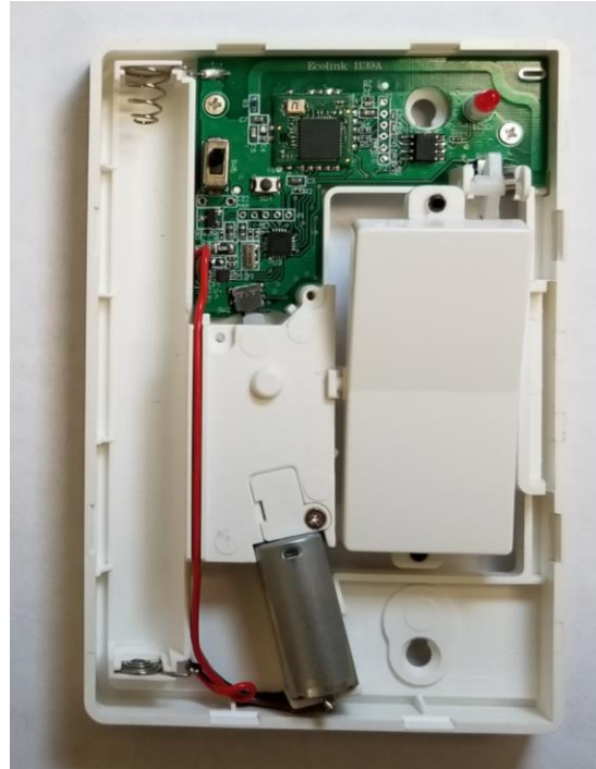
Front inside – front PCBA exposed
