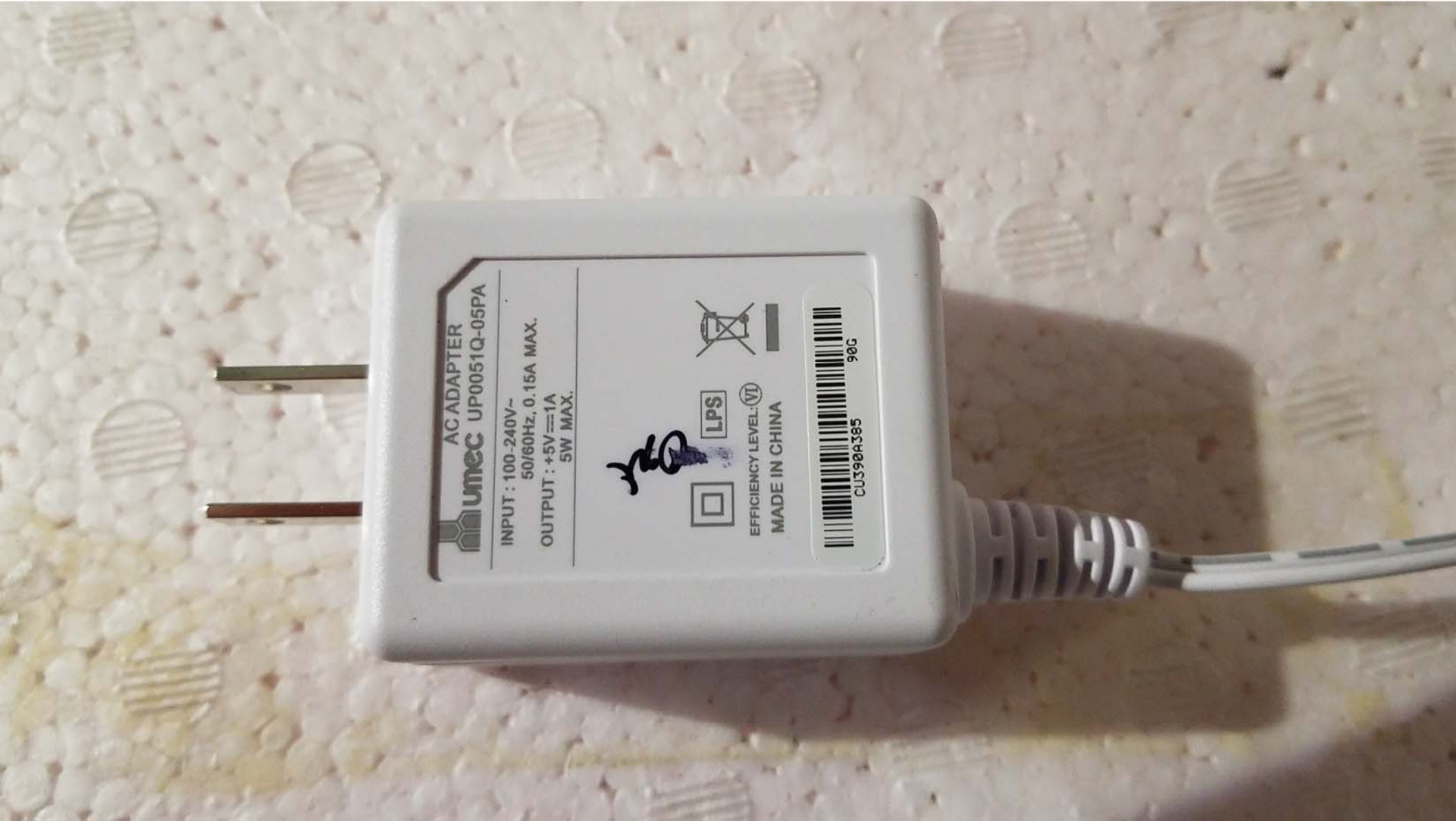
View of the Power Supply for the EUT
