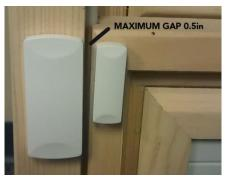
Once your sensor is correctly installed, open and close the door or window. As you open you should hear the bridge beep. Note the bridge will not beep when you close the door.
