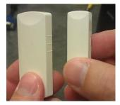
To trigger a learn command from the sensor, touch the magnet to the sensor three times within 2 seconds.
