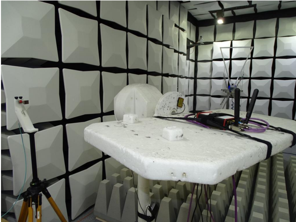
Photo 2: Test setup for radiated measurements (Part 95)
