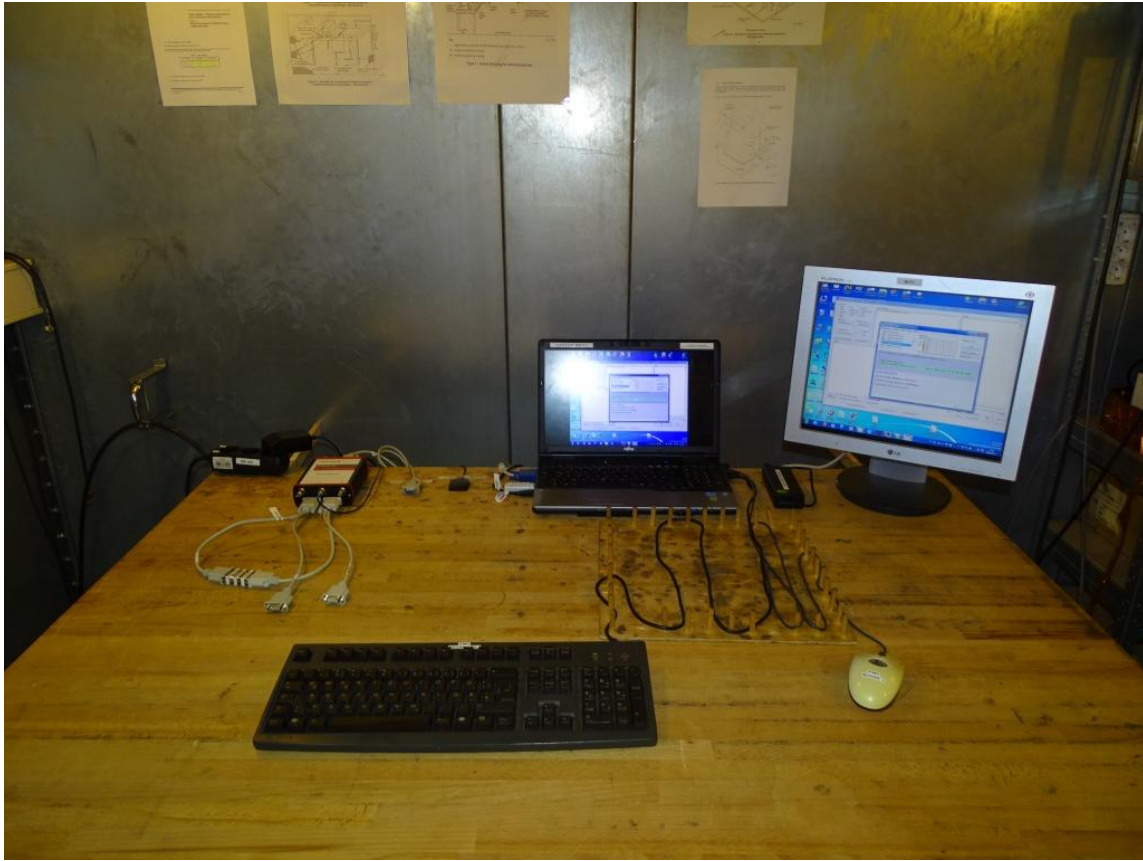
Photo 5: Test setup for conducted measurements (FCC 15B)
