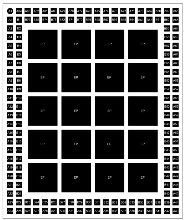
Figure 2: Pin allocation (top view)
