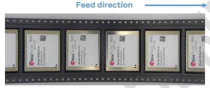
Figure 4: Orientation of VERA-P1 module on tape
