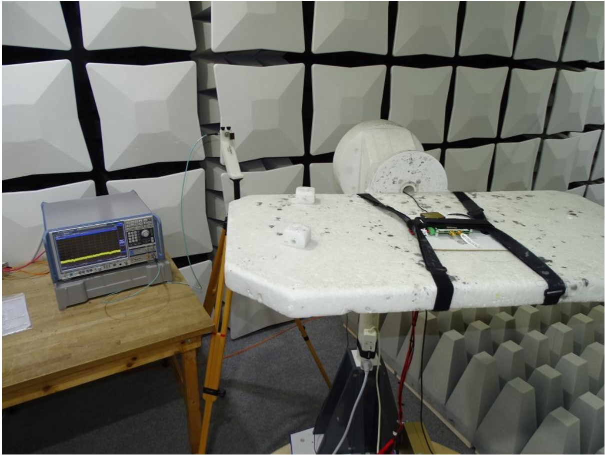
Photo 2: Test setup for radiated measurements (26 - 40 GHz)
