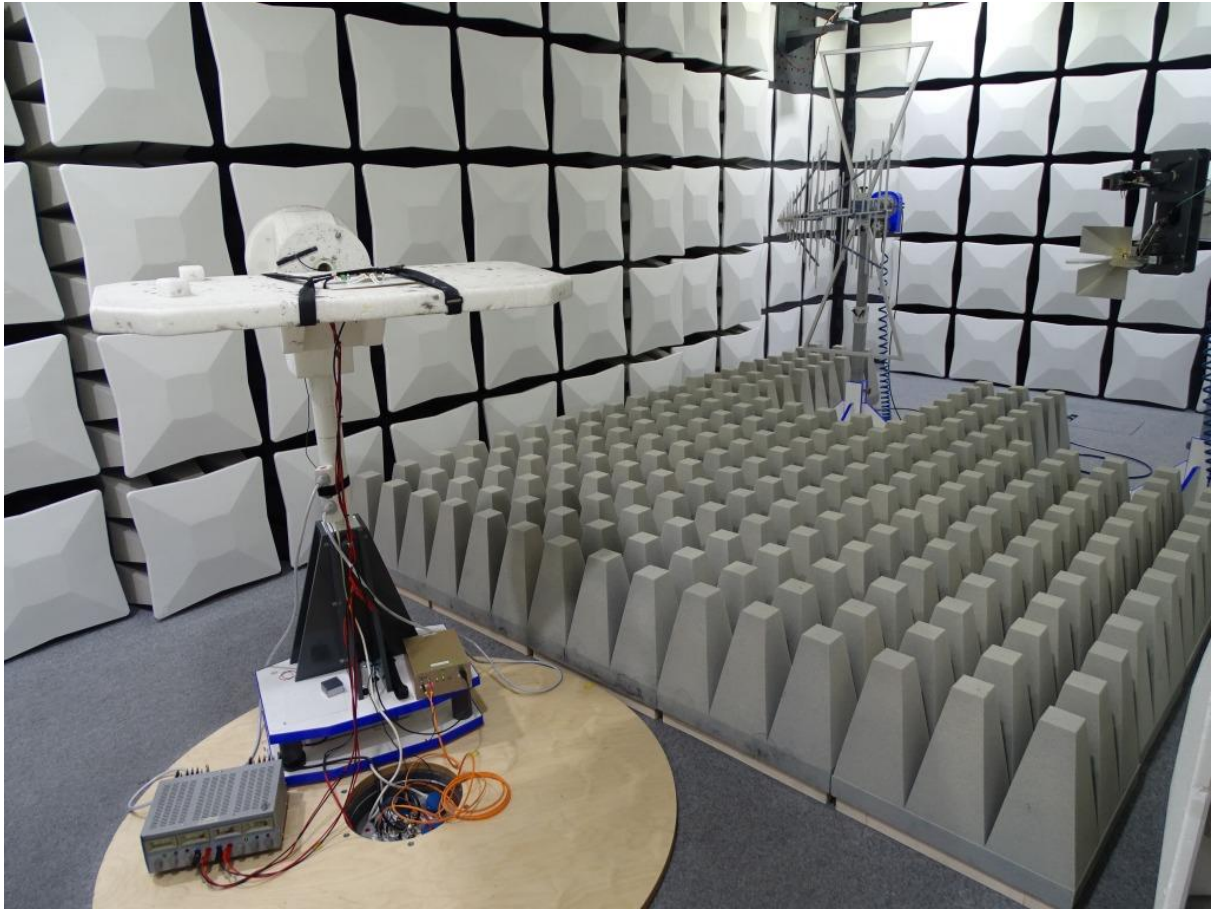
Photo 3: Test setup for radiated measurements above 1 GHz
