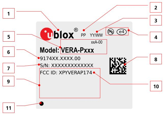
Figure 1: VERA-P1 module series label contents and layout specification
