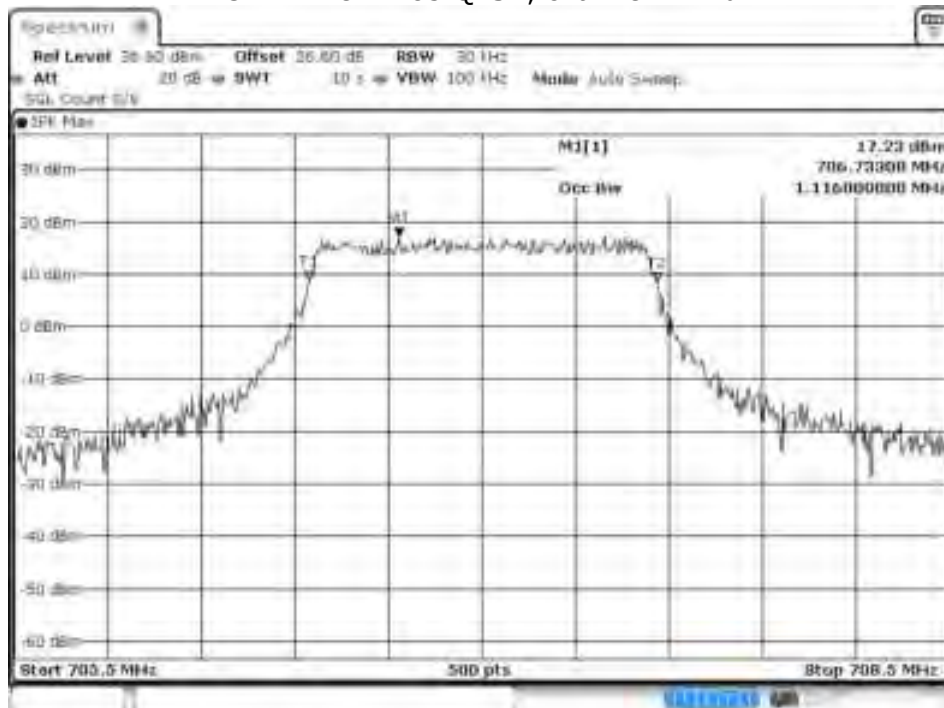
CAT-M1 eFDD85 QPSK, channel = mid
