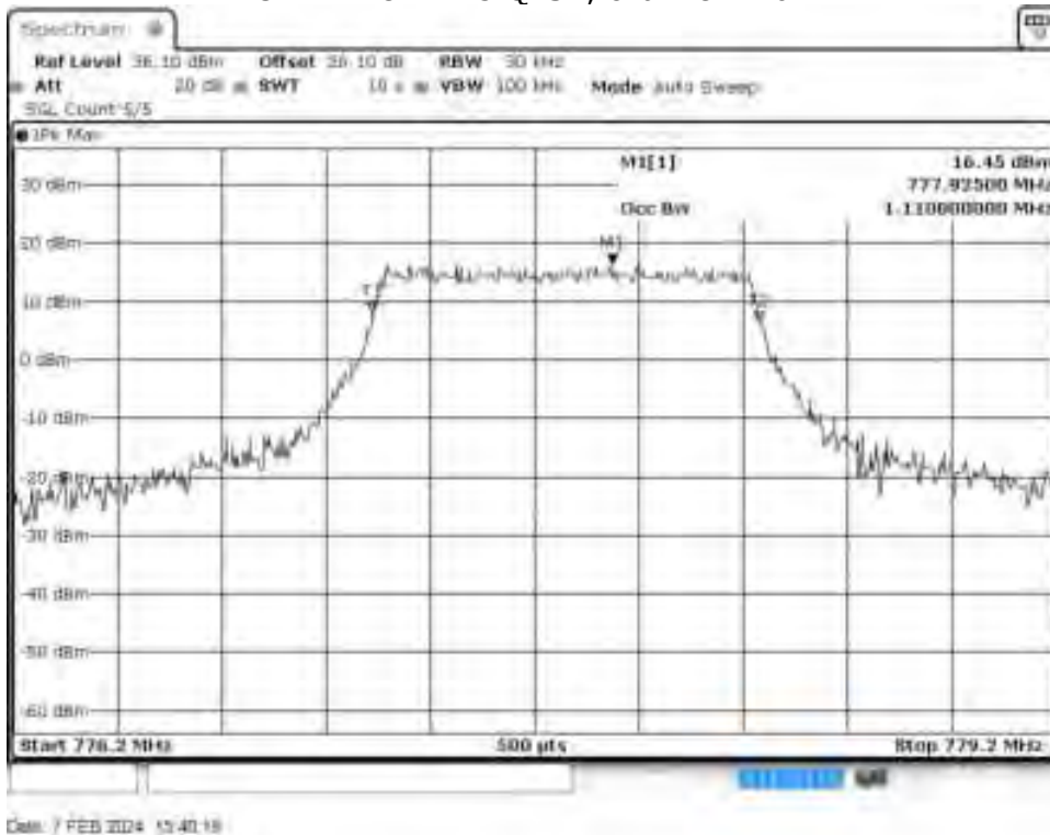
CAT-M1 eFDD13 QPSK, channel = low
