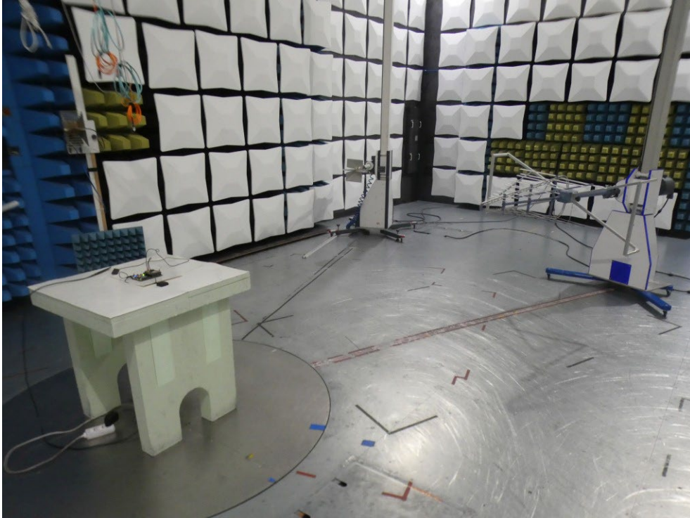
Photo 4: Test setup for radiated measurements below 1GHz
