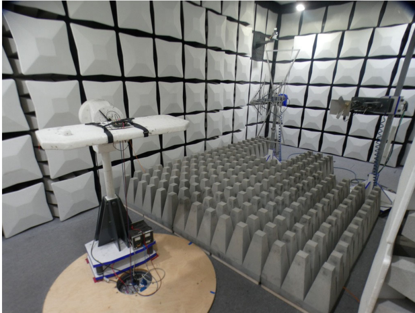
Photo 1: Test setup for radiated measurements above 1GHz
