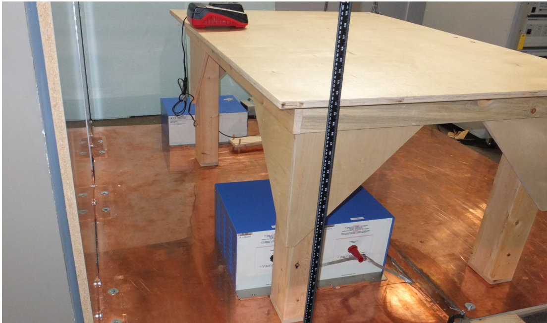
Figure 3.5 - Conducted Emission test setup
