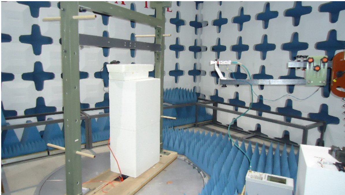
Figure 4.9 - Radiated Emission Test Setup - Side View
