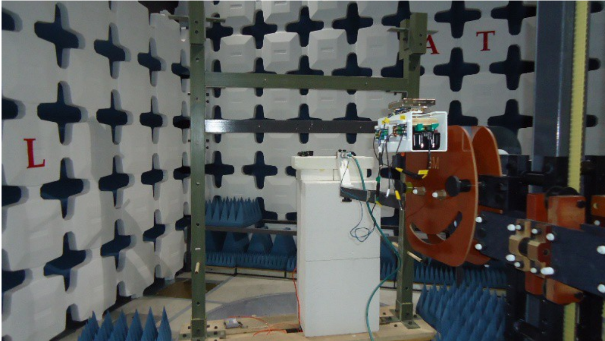
Figure 4.8 - Radiated Emission Test Setup - Front View
