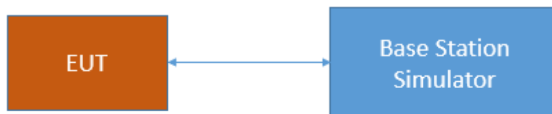
Test Setup FCC Part 22/24/27/90 Cellular; Frequency stability
