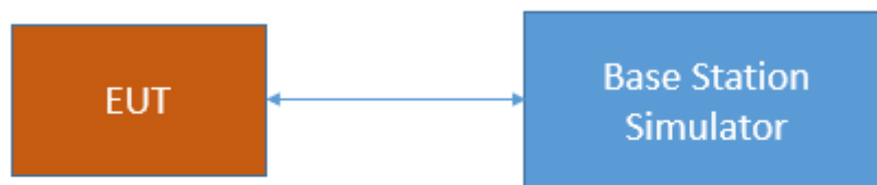
Test Setup FCC Part 22/24/27/90 Cellular; Frequency stability
