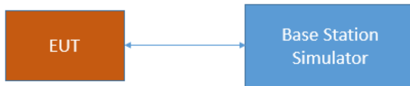
Test Setup FCC Part 22/24/27/90 Cellular; Frequency stability
