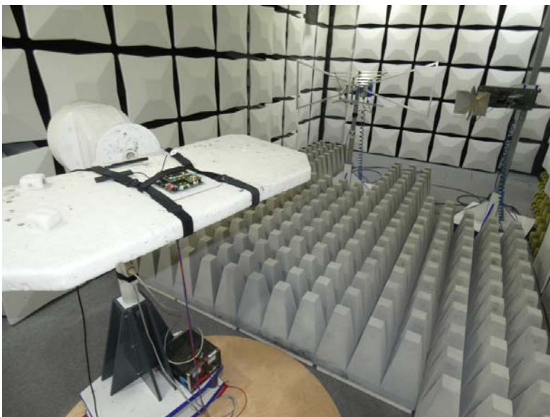
Photo 2: Test setup for radiated measurements (below 1 GHz)
