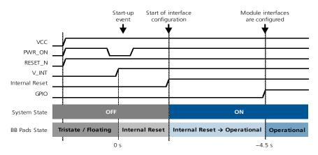
Figure 9: SARA-R4/N4 series switch-on sequence description
