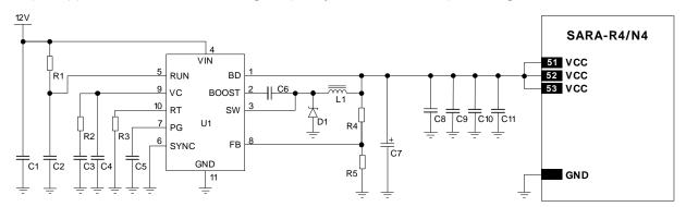
Figure 16: Example of high reliability VCC supply circuit for SARA-R4/N4 series modules, using a step-down regulator
