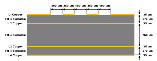
Figure 49: Example of USB line design, with  $Z_0$  close to 90  $\Omega$  and  $Z_{CM}$  close to 30  $\Omega$ , for the described 4-layer board layup
