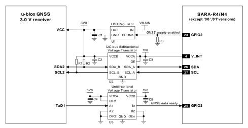
Figure 52: Application circuit for connecting SARA-R4/N4 series modules to u-blox 3.0 V GNSS receivers
