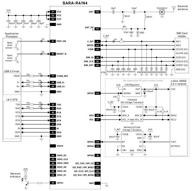
Figure 55: Example of schematic diagram to integrate a SARA-R4/N4 series module using all available interfaces<sup>20</sup>
