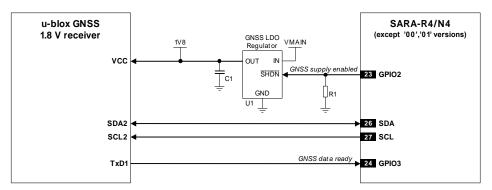
Figure 51: Application circuit for connecting SARA-R4/N4 series modules to u-blox 1.8 V GNSS receivers
