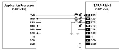
Figure 46: UART interface application circuit with a 3-wire link in the DTE/DCE serial communication (1.8V DTE)
