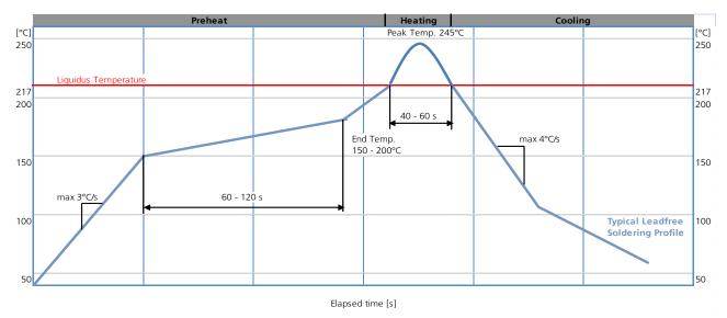
Figure 56: Recommended soldering profile
