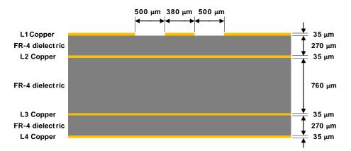
Figure 32: Example of 50 Ω coplanar waveguide transmission line design for the described 4-layer board layup
