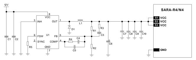
Figure 18: Example of low cost VCC supply circuit for SARA-R4/N4 series modules, using a step-down regulator
