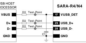
Figure 48: USB Interface application circuits
