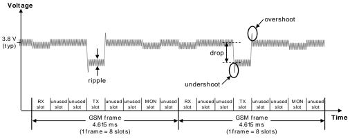
Figure 6: Description of the VCC voltage profile versus time during a 2G single-slot call (1 TX slot, 1 RX slot)
