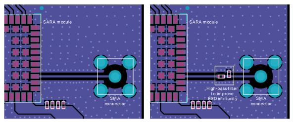
Figure 34: Example of circuit and layout for antenna RF circuits on the application board
