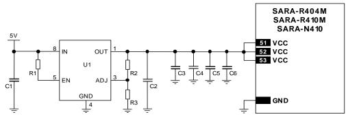
Figure 20: Example of high reliability VCC supply circuit for SARA-R404M /-R410M /-N410, using an LDO linear regulator
