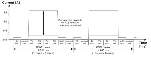
Figure 7: VCC current consumption profile versus time during a GPRS multi-slot class 12 connection (4 TX slots, 1 RX slot)
