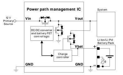
Figure 23: Charger / regulator with integrated power path management circuit block diagram
