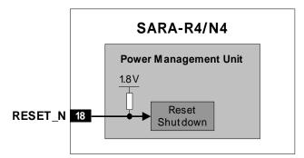
Figure 12: RESET\_N input description
