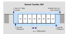
Figure 13: Description of UART 8N1 frame format (8 data bits, no parity, 1 stop bit)
