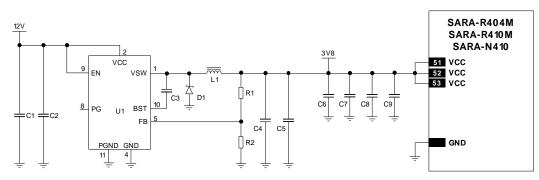
Figure 17: Example of high reliability VCC supply circuit for SARA-R404M /-R410M /-N410, using a step-down regulator
