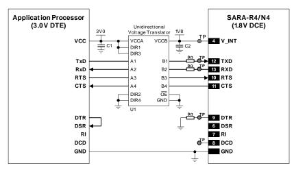
Figure 45: UART interface application circuit with a partial V.24 link (5-wire) in DTE/DCE serial communication (3.0 V DTE)
