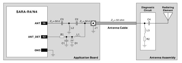
Figure 35: Suggested schematic for antenna detection circuit on application PCB and diagnostic circuit on antenna assembly
