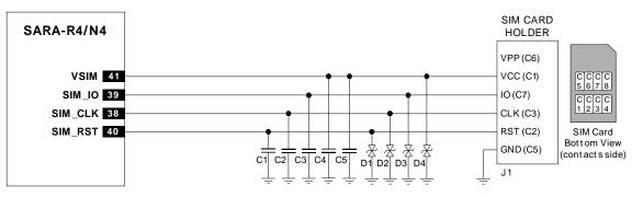
Figure 37: Application circuits for the connection to a single removable SIM card, with SIM detection not implemented
