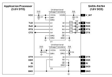
Figure 43: UART interface application circuit with partial V.24 link (6-wire) in DTE/DCE serial communication (3.0 V DTE)
