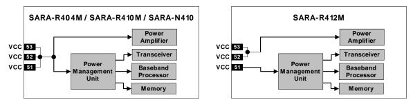
Figure 3: Block diagram of SARA-R4/N4 series modules' internal VCC supply routing
