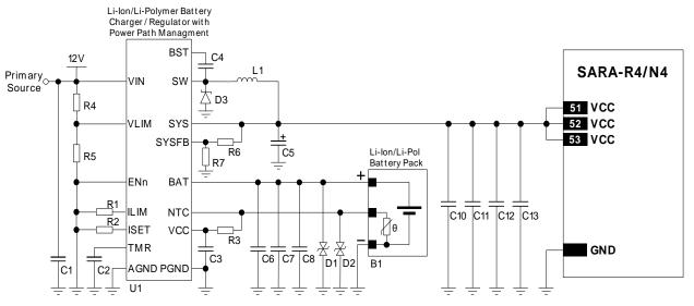
Figure 24: Li-Ion (or Li-Polymer) battery charging and power path management application circuit
