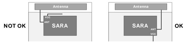
Figure 28: VCC line routing guideline for designs integrating an embedded antenna
