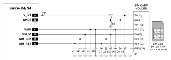
Figure 39: Application circuit for the connection to a single removable SIM card, with SIM detection implemented
