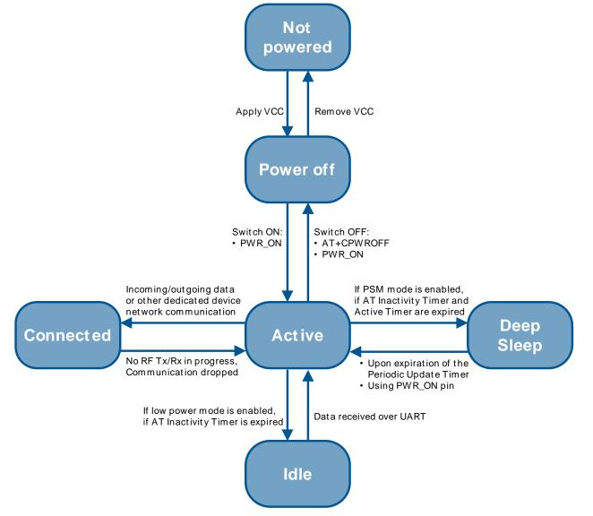
Figure 2 describes the transition between the different operating modes.
