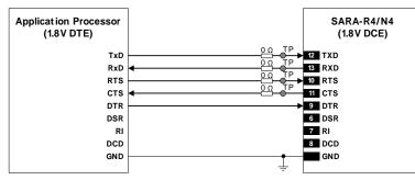
Figure 42: UART interface application circuit with partial V.24 link (6-wire) in the DTE/DCE serial communication (1.8 V DTE)
