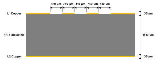
Figure 50: Example of USB line design, with  $Z_0$  close to 90  $\Omega$  and  $Z_{CM}$  close to 30  $\Omega$ , for the described 2-layer board layup
