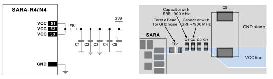
Figure 27: Suggested design to reduce ripple / noise on VCC, highly recommended when using an integrated antenna
