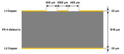
Figure 33: Example of 50 Ω coplanar waveguide transmission line design for the described 2-layer board layup
