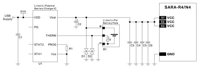
Figure 22: Li-Ion (or Li-Polymer) battery charging application circuit
