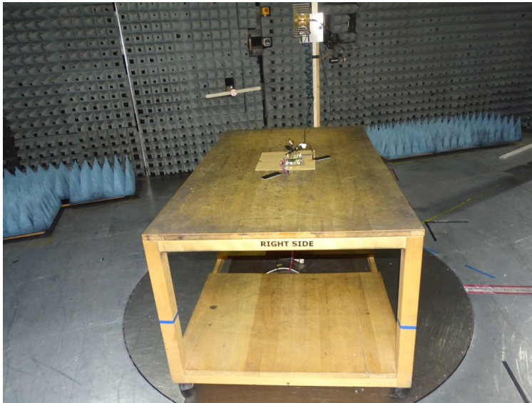
Photo 1: Test setup for radiated measurements
